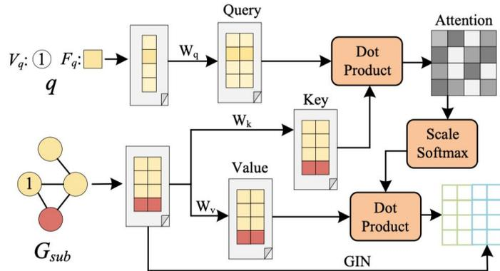
Figure 6: Illustration of Cross Attention Encoder
