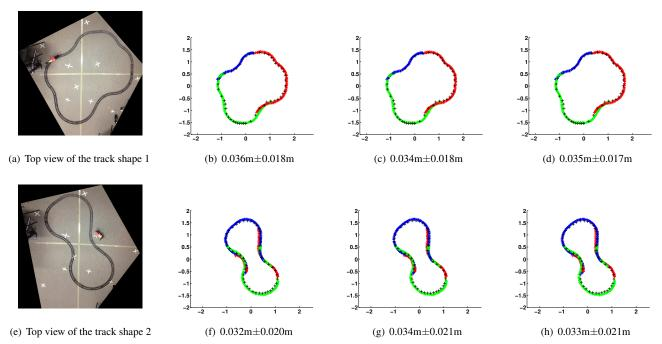
Figure 10. Target tracking experiment set-up and results. The black cross are the ground truth and the other different colour cross represent the results from different camera nodes.
