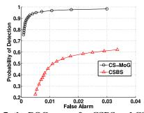
Figure 7. the ROC curves for CSBS and CS-MoG.
