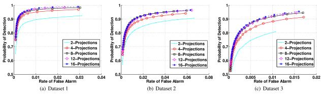
Figure 3. ROC curves for CS-MoG-Balance for different number of projections for the three datasets.
