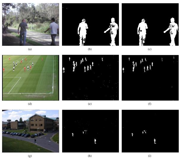
Figure 5. Sample background subtraction outputs for MoG (middle column) and CS-MoG-Balanced (rightmost column). The i-th (i = 1, 2, 3) row contains the results from the i-th dataset. The original frames are in the leftmost column.
