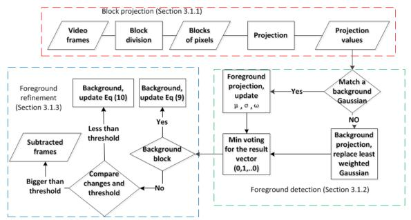
Figure 1. Flow chart of the Algorithm. Different components are grouped by dashed frames in different color
