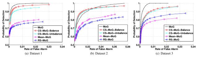
Figure 4. ROC curves for different MoG-based methods for the three datasets.
