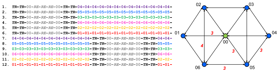
Fig. 8 Scheduling solution for Instance 1a ( T_E = 18 , T_R = 4 , T = 88 ), with Problem Network 1 shown on the right-hand side. This solution is cyclic over a period of 22 time units, is naturally integer at the root node and exhibits a block scheduling structure. A total of 12 vessels are required for complete patrol coverage, with replenishment at port synchronized within the two equal groupings of the fleet. Exactly two vessels are needed to cover each region, with one time unit of overlapping patrol incurred per handover
