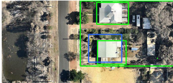
Figure 3.2: An example of annotations produced by 3 crowd workers for a single image, blue annotations for collapsed buildings, green for intact buildings.
