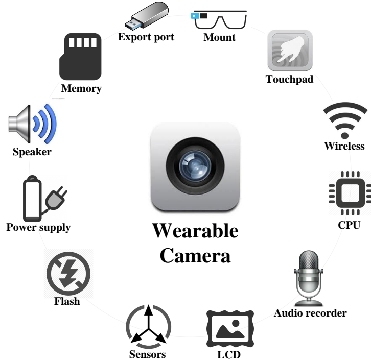
(a) The main hardware components for a wearable lifelogger. Camera, memory, export port, audio player/recorder, touchpad, battery/charger and screen are the main usual components in any WVL.
