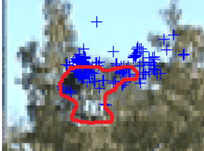
Figure 3.1: Particles, which are scattering chaotically are drawn by little blue crossings. The estimated position for the helicopter is centered by the green ellipse. The ground truth of the boundary of tracked object is highlighted by the red line. This figure is cropped out from the video sequence data when the helicopter is in front of brown leaves. It is very difficult to recognize the helicopter even for human beings.
