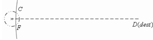
Fig. 5. As L \gg R , the arc \widehat{CF} can be approximated as line CF
