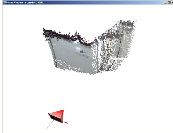
Figure 4: An example of a snap. Red arrow denotes the robot's orientation.
