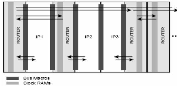
**Figure 5: Wormhole Routing**
