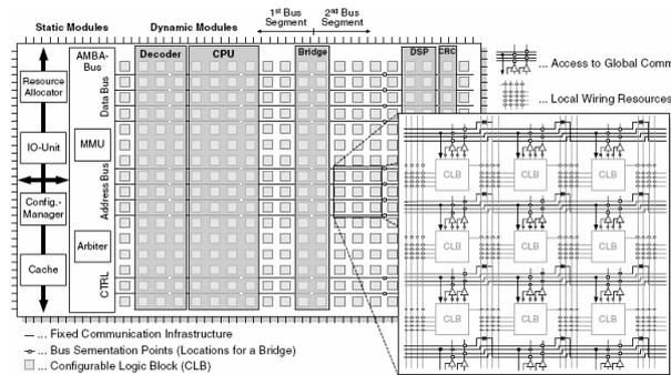
**Figure 3: 1-D Relocatable Modules**
