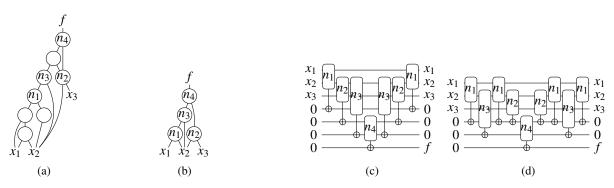
Figure 3: (a) a three-input multi-level logic network performing the Booelan function f; (b) an example of a 2-LUT network for f; (c) the reversible circuit for the 2-LUT network obtained using the Bennett clean-up strategy; (d) the reversible circuit for the 2-LUT network obtained using the quantum garbage management clean-up strategy [11].
