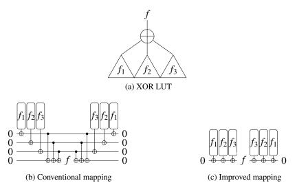
Figure 5: Mapping LUTs that represent the XOR function
