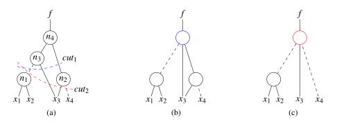
Figure 1: (a) an AIG graph performing the function  $f = (\overline{x}_1 + \overline{x}_2)x_3\overline{x}_4$  with two possible 3-feasible cuts; (b) 3-LUT network generated by *cut*<sub>1</sub>; (c) 3-LUT network generated by *cut*<sub>2</sub>.
