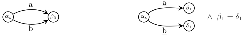
Figure 7: Two abstractions drawn from the combined abstract domain \mathbb{H}^\sharp \rightrightarrows \mathbb{N}^\sharp that have equivalent concretizations but with non-isomorphic sets of symbolic variables.
