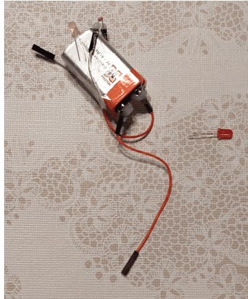
Figure 3: A small lamp mounted on a battery with cables. It can be attached to a moving object by a glue tape.
