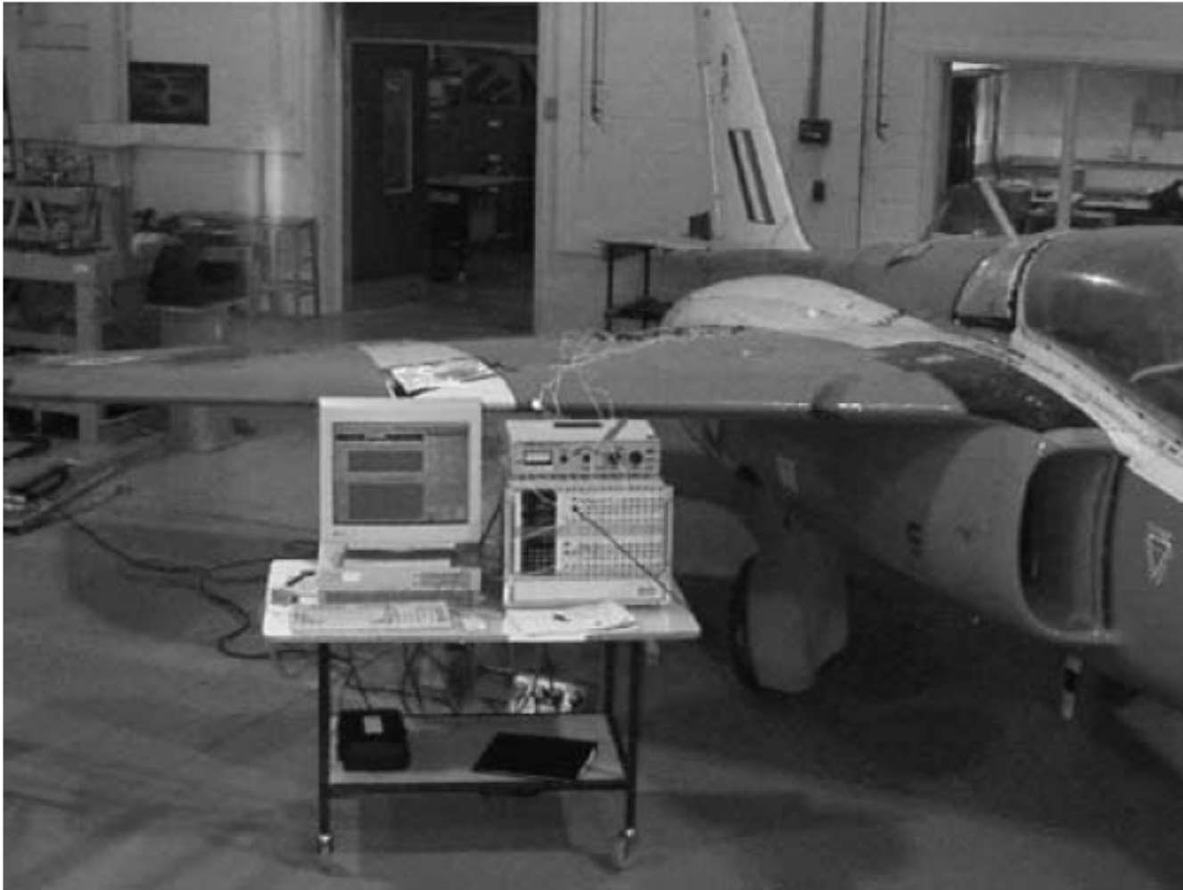
Figure 2. Gnat aircraft and acquisition system.
