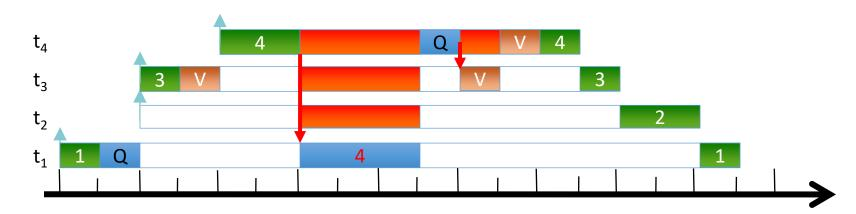
If t<sub>1</sub> blocks on a resource held by t<sub>2</sub>, and P<sub>1</sub>>P<sub>2</sub>, then t<sub>2</sub> is temporarily given priority P<sub>1</sub> – when t₁ releases the resource, its priority reverts to P₂ Long blocking **Transitive** chains! Inheritance  $\mathsf{t}_{5}$  $t_3$  $t_2$
