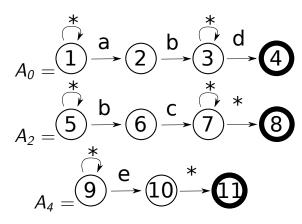
$A_0$  is the automaton for the "main" XPath expression. The other  $A_i$ automata correspond to the filter which must be checked for state *i* of automaton  $A_0$ .
