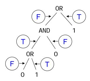
$\begin{array}{c} 0() \rightarrow F \\ 1() \rightarrow T \\ OR(F,F) \rightarrow F \\ OR(F,T) \rightarrow T \\ \dots \\ AND(T,F) \rightarrow F \end{array}$
