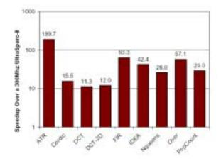
i Speedup for 8-bit Pes, 8 registers/PE, 128-bit wide stripes (stages)
