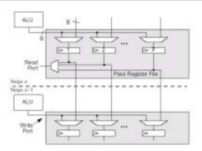
Provides efficient (registered) interstage connections; ALU output can write to any of P registers otherwise register is loaded from previous stage
