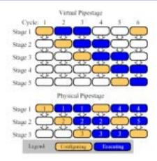
This diagram illustrates the process of virtualizing a five-stage pipeline on a three-stage device
