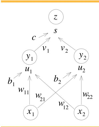
$u_{1} = b_{1} + w_{11}x_{1} + w_{12}x_{2}$   $y_{1} = g(u_{1})$   $s = c + v_{1}y_{1} + v_{2}y_{2}$  z = g(s) $E = \frac{1}{2}\sum(z-t)^{2}$
