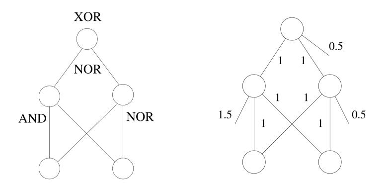
Given an explicit logical function, we can design a multi-layer neural network by hand to compute that function. But, if we are just given a set of training data, can we train a multi-layer network to fit these data?
