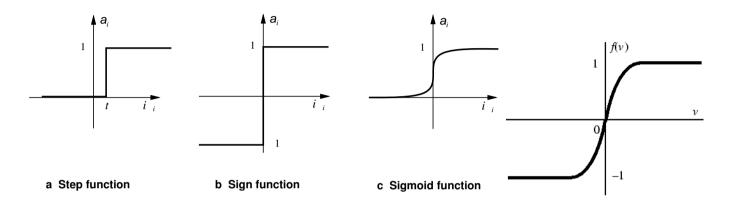
Replace the (discontinuous) step function with a differentiable function, such as the sigmoid:
