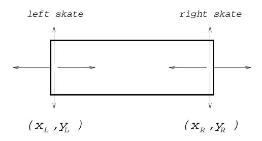
a skate at each end of the vehicle with which it can push on the rink in two independent directions
