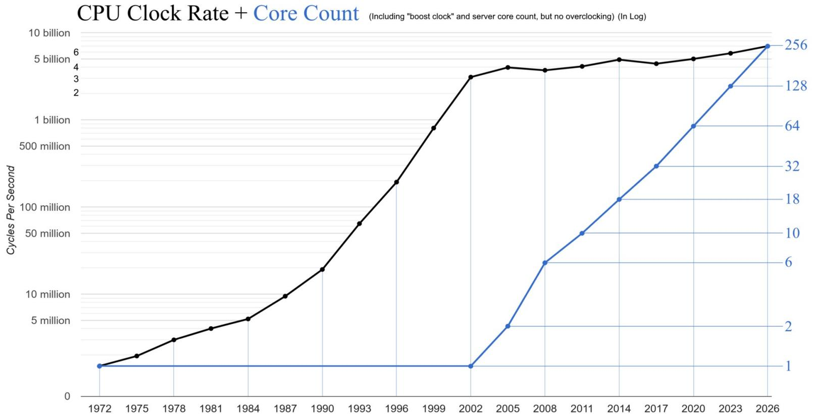
Source: <https://www.singularity.com/charts/page61.html> 1976- 1998 "Microprocessor clockspeed" (modified) | 1999-2026 Manufacturer specifications
