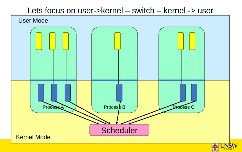
Running in user mode, SP points to user-level stack (not shown on slide)
