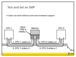
Test-and-Set on SMP A solution: • Hardware blocks all other CPUs from accessing the bus during the TSL instruction to prevent memory accesses by any other CPU. • TSL has mutually exclusive access to memory for duration of instruction. Word CPU 1 CPU 2 Memory 1000 is initially 0 1. CPU 1 reads a 0 2. CPU 2 reads a 0 4. CPU 2 writes a 1 3. CPU 1 writes a 1 34
