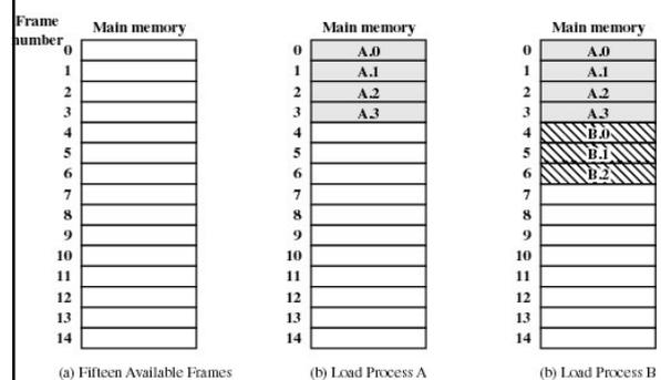
Figure 7.9 Assignment of Process Pages to Free Frames
