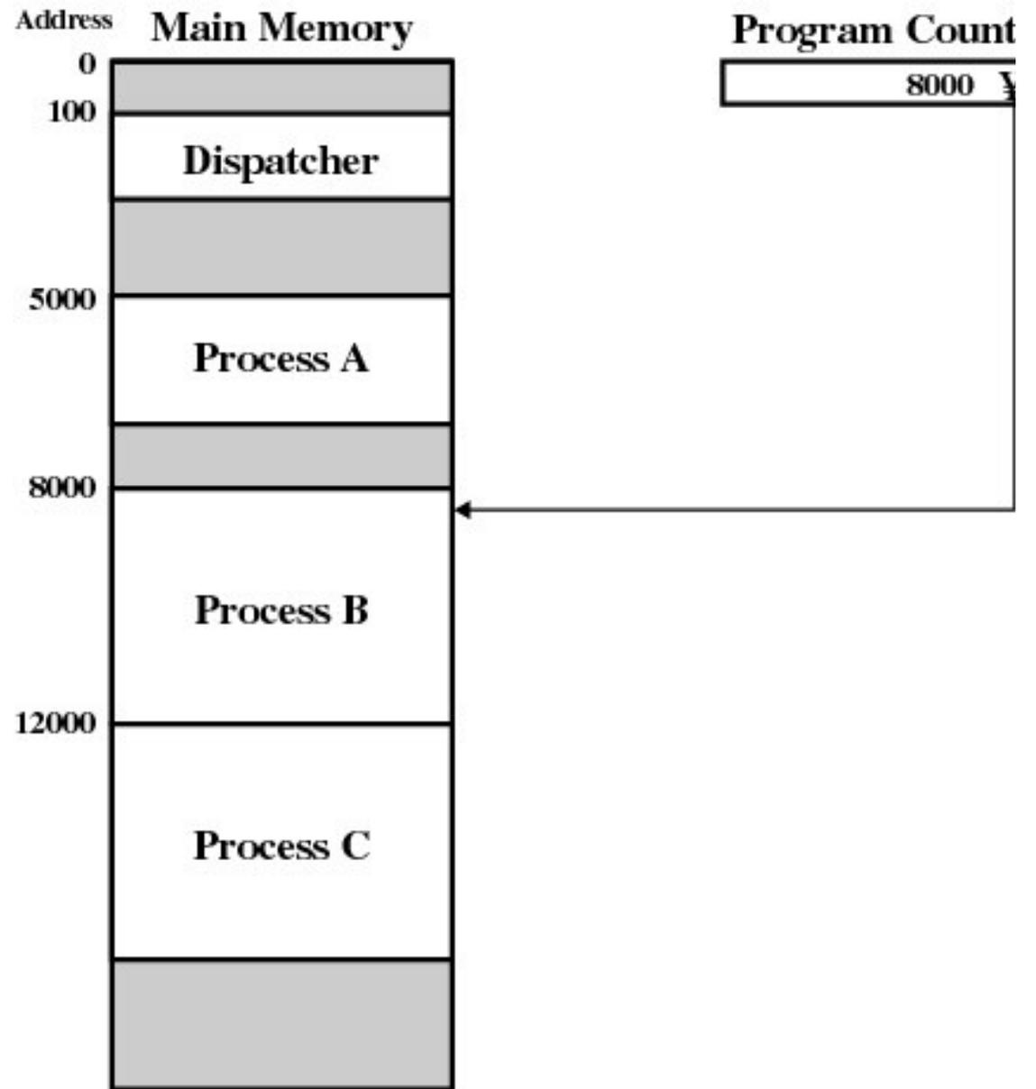
Figure 3.1 Snapshot of Example Execution (Figure 3 at Instruction Cycle 13
