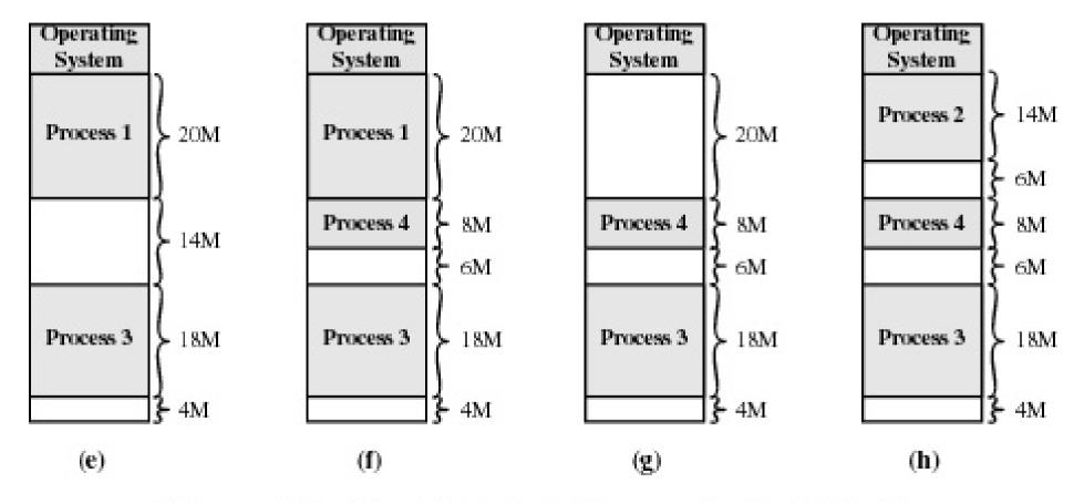
Figure 7.4 The Effect of Dynamic Partitioning
