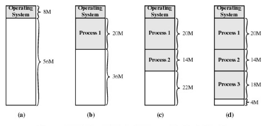
Figure 7.4 The Effect of Dynamic Partitioning
