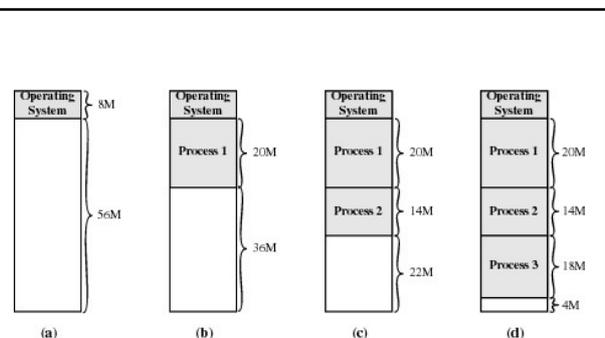
Figure 7.4 The Effect of Dynamic Partitioning
