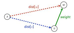
In edge relaxation, we take the shortest known path from s to v and extend it using edge (v, w, weight) to create a new path from s to w.
