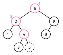
Balance must be checked at 4, then at 2, then at 6
