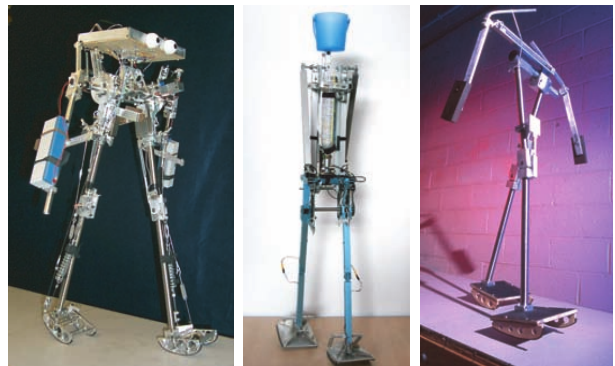
Figure 1.1: An assortment of passive-dynamic walkers developed at Cornell. The first robot is powered at the ankles, the second is powered at the hips, and the last is entirely passive.
