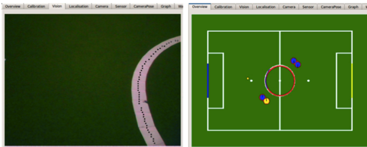
Figure 2.5: The RANSAC algorithm detecting the centre circle even when only a part of it was visible [10].
