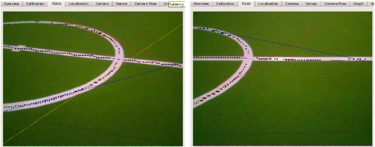
Figure 2.7: The RANSAC algorithm detecting line segments in the centre circle [10].
