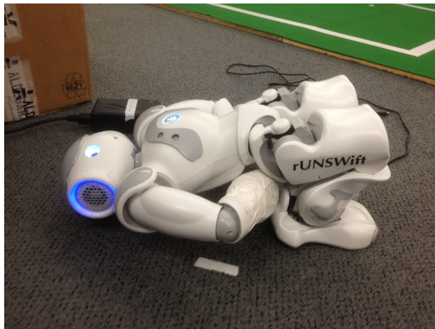
Figure 4.5: Legs are curled down to create space under the back for the arms to shift in and support the weight of the robot.
