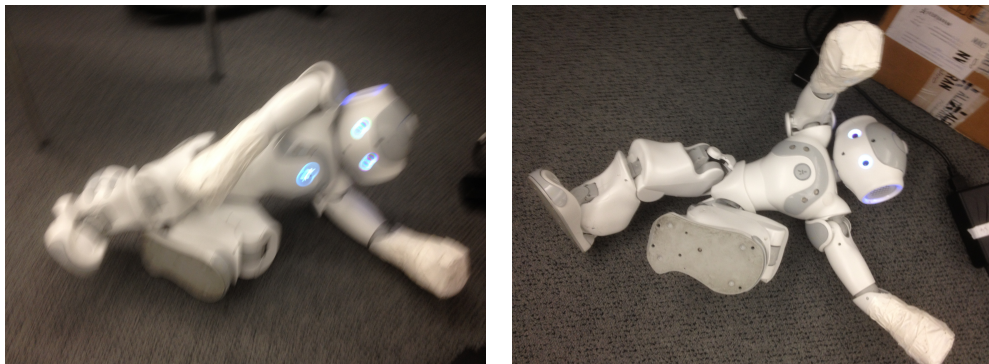
Figure 5.4: The dive motion rolling the robot on its back.
