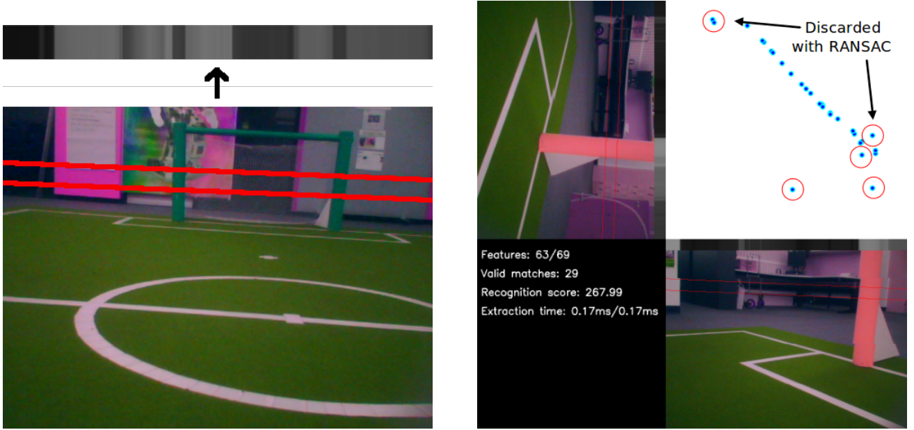
Fig. 3. Left: Image captured by the Nao robot showing superimposed 30 pixel horizon band in red, and the extracted grey-scale horizon pixels at the top of the image. Right: Matching 1D SURF features between two similar images, with outliers discarded using RANSAC.
