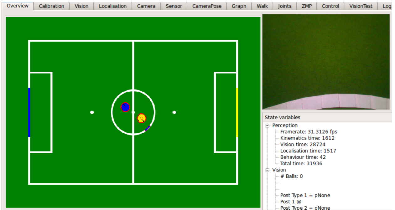
Figure 4.8: The segment is classified as a short line as opposed to a piece of the centre circle
