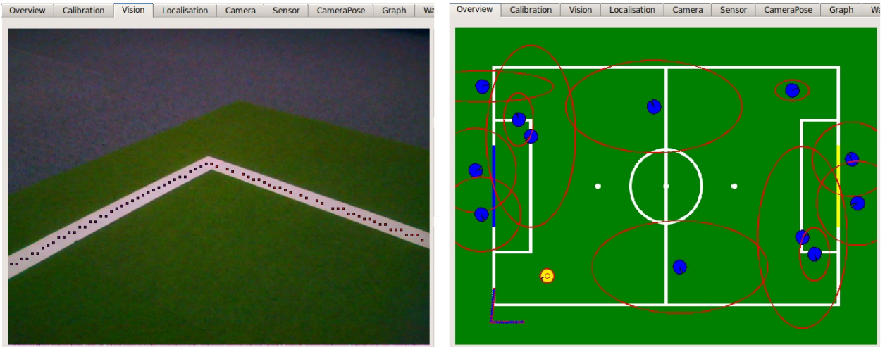
Figure 4.4: Line detection as shown by the vision tab (left) and the overview tab (right)
