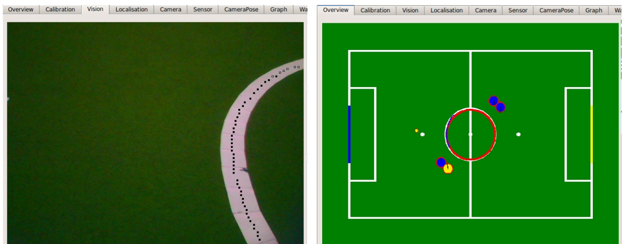
Figure 4.5: Circle detection as shown by the vision tab (left) and the overview tab (right)
