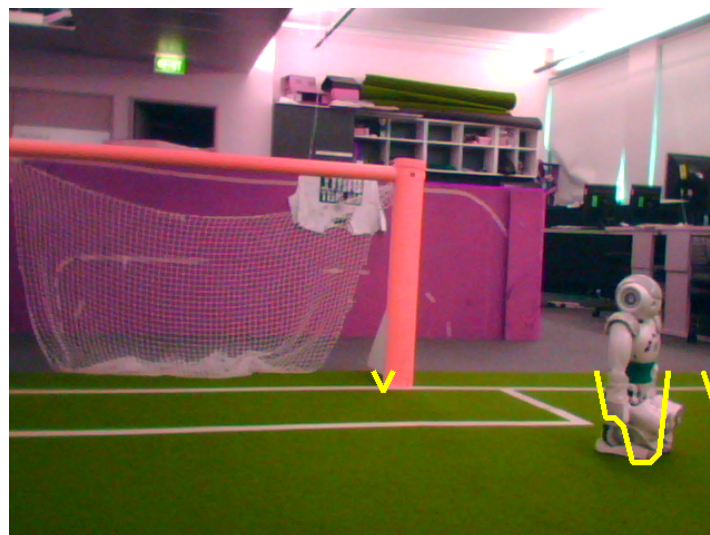
Figure 3.12: The end result after first two steps of the algorithm. Despite its best effort, there are still unwanted indentations in the visual frame.
