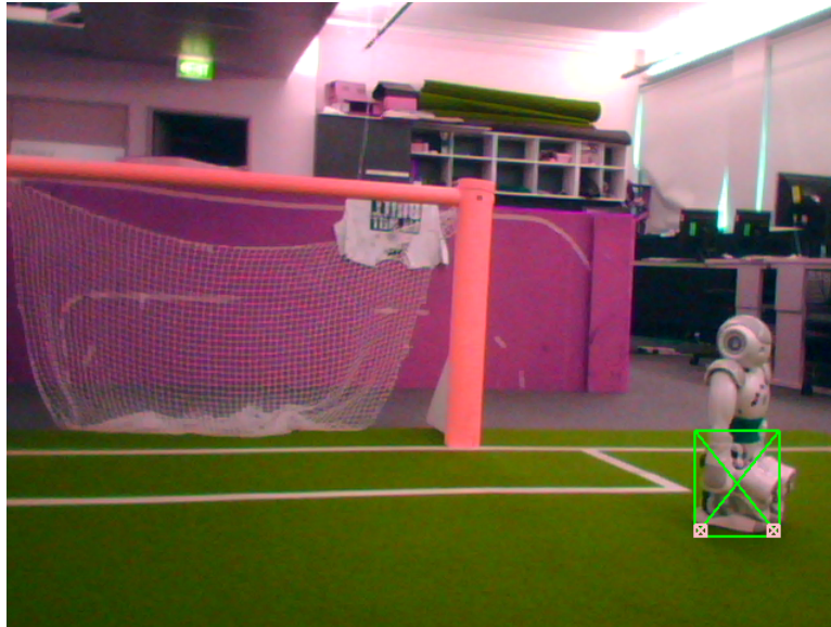
Figure 3.21: Width estimation that demonstrates the two points used when attempting to calculate the straight line distance, in other words, the width of the robot.
