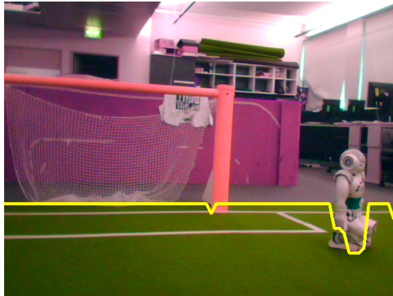
Figure 3.9: The generated indentation after the first search process shows the indentation created from the field edge. The indentation is similar to how it was visualised in the concept section.
