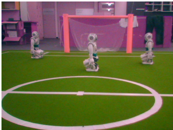
Figure 2.4: The raw image of obstructed waistband. The waistband is still visible in this image as the image is in much a higher resolution than the saliency image.
