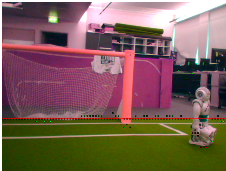
Figure 3.8: The generation of candidate robot points that shows the first execution step of the algorithm. The green points are the recycled field edge points, red line is the edge line and the red points are the candidate robot points generated.
