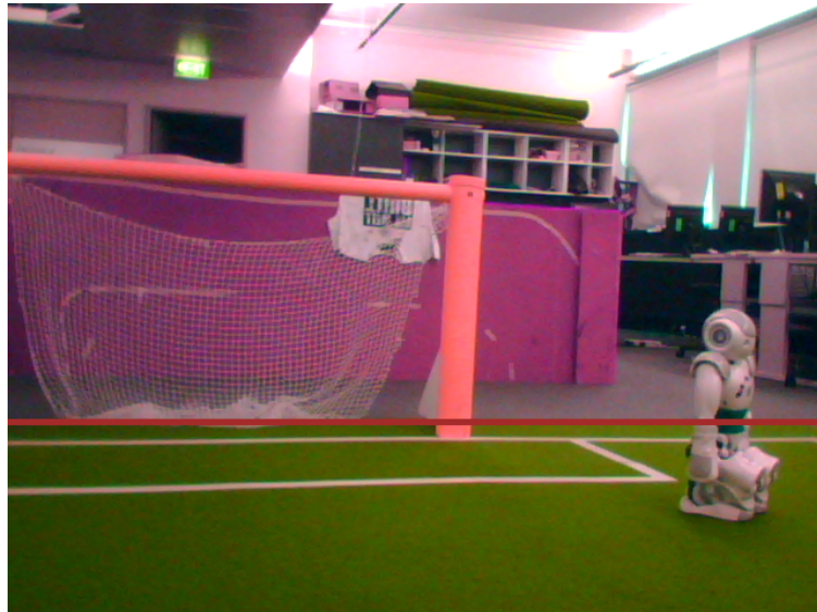
Figure 3.4: Result of Field Edge Detection. The brown line represents the detected edge of the field.
