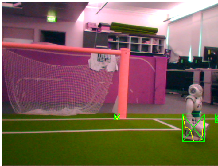
Figure 3.13: Bounding of points into boxes that shows how a region is created based on the candidate points generated from the first stage.
