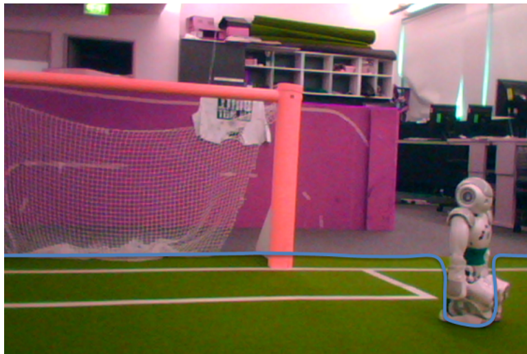
Figure 3.1: Concept of robot detection that shows the basic premise on how it works. The blue line is the line generated from running the steps above. Notice the indentation near the robot.
