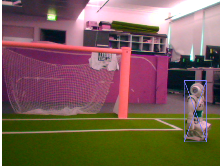
Figure 3.20: Height estimation correction demonstrates how an incorrectly estimated height can be corrected.
