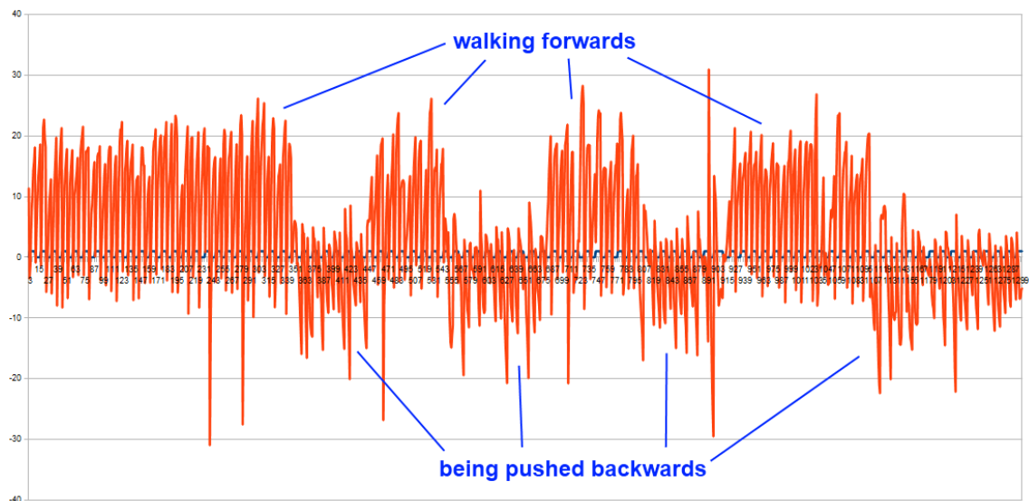
Figure 5.6.: The different regions show when the robot walks forwards and when it is following the chairs direction walking backwards.
