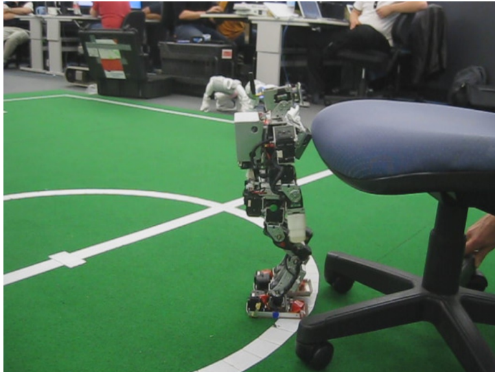
Figure 5.5.: The robot colliding with a chair. The robot being the weaker opponent has to give in and follow the chairs direction.
