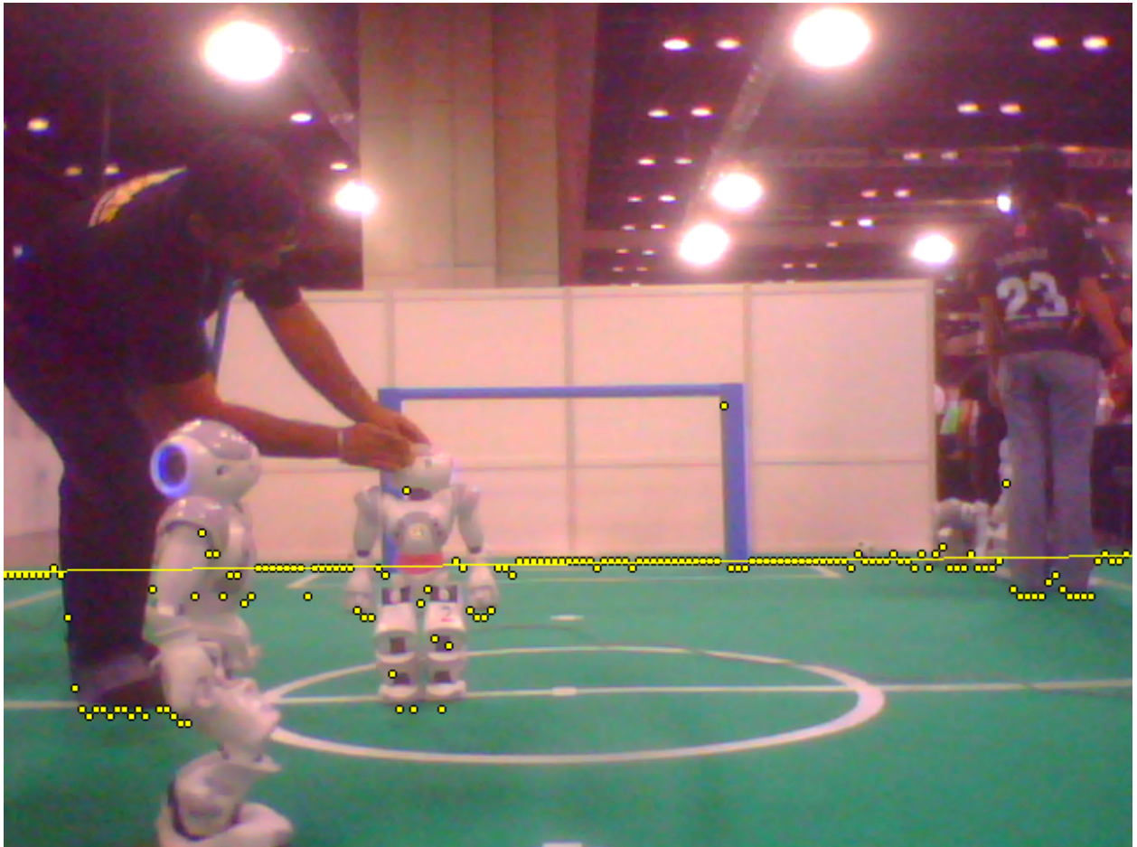
Figure 4.5: Line found by performing RANSAC on the candidate points
