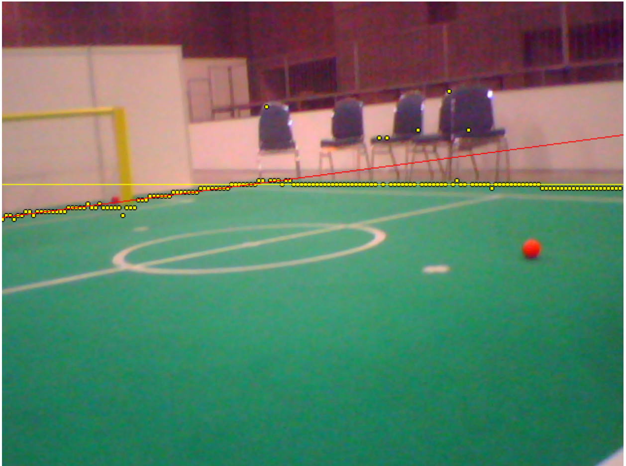
Figure 4.6: Lines found by performing RANSAC twice on the candidate points
