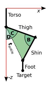
Figure 2.8: Side View of the Leg.
