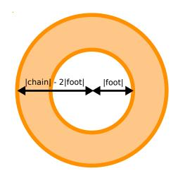
Figure 2.3: A two dimensional cross section of the reachable sphere where all orientations are reachable.
