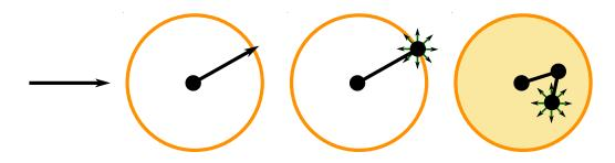
Figure 2.2: Progression of reachable targets as joints are added to the chain.
