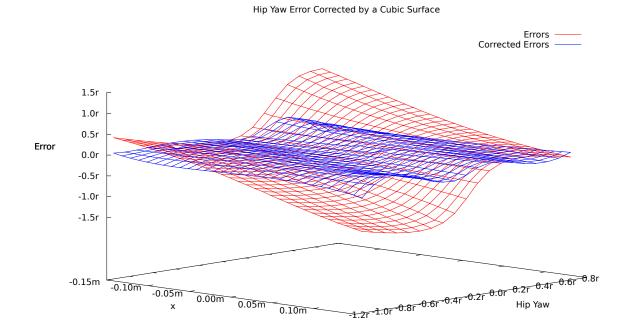
Figure A.1: Yaw error corrected by a cubic surface.
