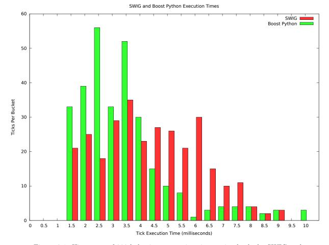
Figure 3.1: Histogram of 300 behaviour execution times using both the SWIG and boost::python python bridges. Results are grouped into 0.5 millisecond buckets; faster execution times will result in a shift towards the left of the graph.
