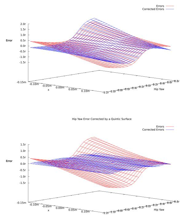
Figure 2.13: Error surface corrected by multiplying the hip yaw by  $1 + \tanh(\operatorname{atan2}(x, -z))$  (top) and subtracting a quintic surface(bottom)
