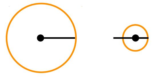
Figure 2.1: An optimally placed joint (left) at the chain origin allows the foot to reach a large circle of targets. A suboptimal placement (right) in the middle of the chain results in a smaller range of possible targets.
