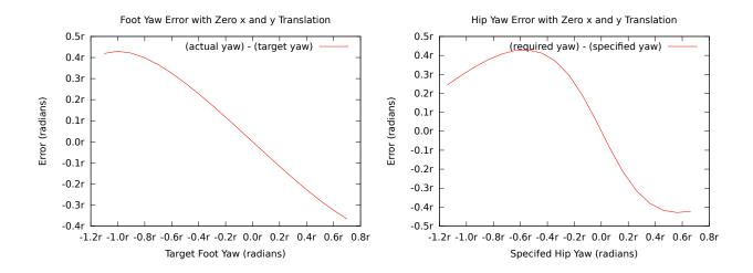
Figure 2.10: Yaw error when the foot is directly below the hip. The left plot shows the error between the target and actual foot yaw. The right plot shows the error between the hip yaw specified by our solution and the correct hip yaw required to reach the users target.
