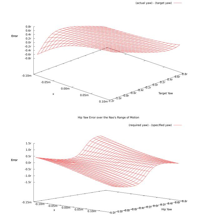
Figure 2.12: Yaw error with respect to target yaw and x translation. The top plot shows the error between the target and actual foot yaw. The bottom plot shows the error between the hip yaw specified by our solution and the correct hip yaw required to reach the users target.
