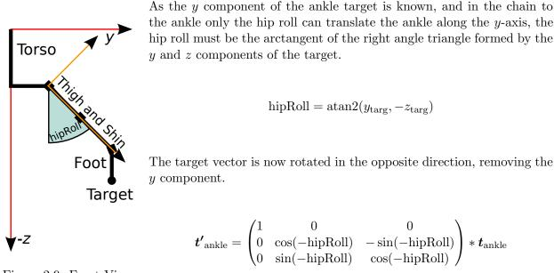
Figure 2.9: Front View of the Leg.
