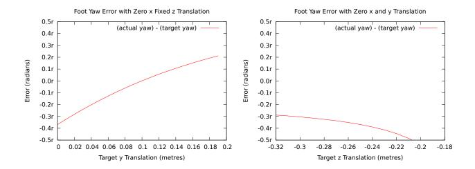
Figure 2.11: Yaw error with respect to y (left) and z (right) translation with target yaw fixed at 45 degrees. 45 degrees is where the error is most prevalent.
