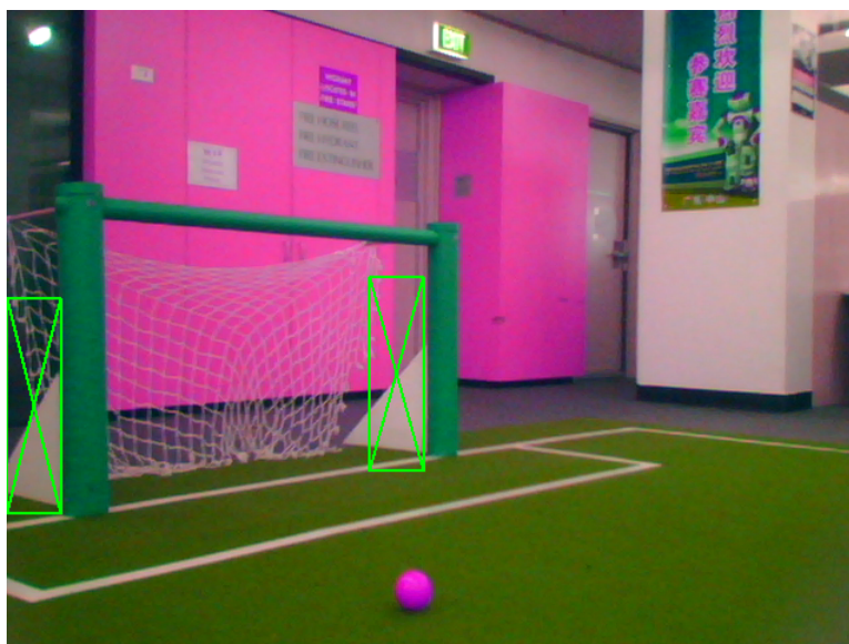
Figure 3.30: The white triangle behind goal posts being incorrectly detected.
