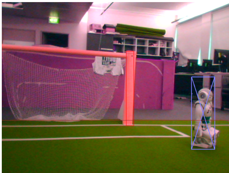
Figure 3.19: Incorrect height estimation where the estimated height is well above the robot.
