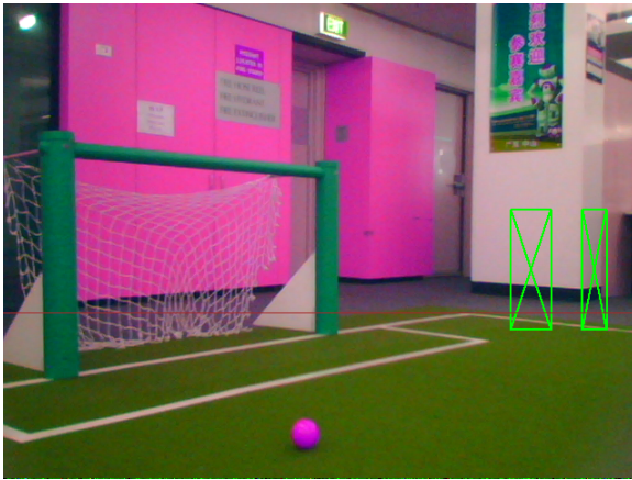
Figure 3.33: Mis-detection when the background colour is white in raw image.
