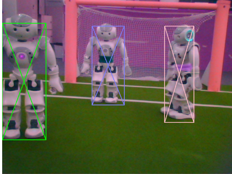
Figure 6.2: One of the test scenario in testing the robot filter. This image contains three different robots each with a different configuration of the waistbands.
