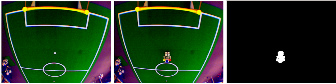
Figure 2: Background image (left). Current camera image (middle). The result of subtraction in threshold image (right).
