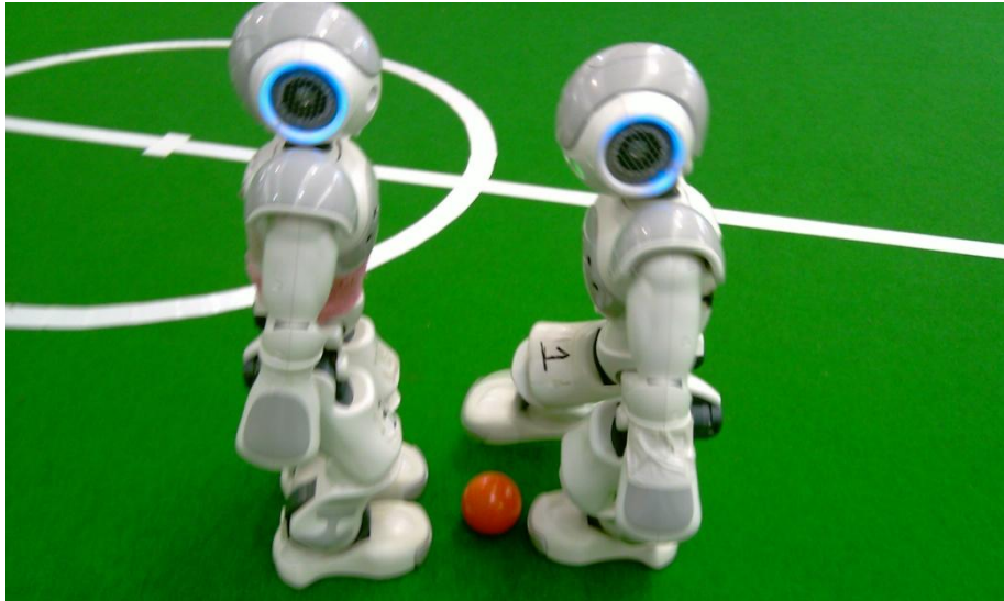
Figure 3: Aldebaran Nao performing a ball stealing manoeuvre – a left side kick.
