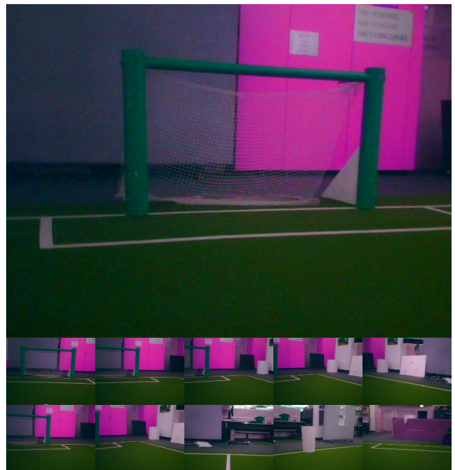
Fig. 14. Successful matching of the first image with the robot placed further away from the goal posts. The table depicts matching scores for the top image against the 10 images tiled in the lower frame. The threshold for images to be considered a match is 200.
