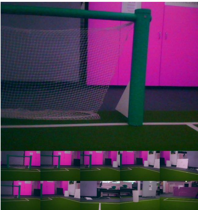
Fig. 12. Successful matching of the first image from a different angle (sideways translation of the robot to its right). The table depicts matching scores for the top image against the 10 images tiled in the lower frame. The threshold for images to be considered a match is 200.
