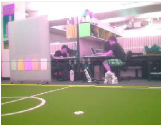
Fig. 1. Image taken from the Nao camera showing superimposed horizon line as determined by robot kinematics.
