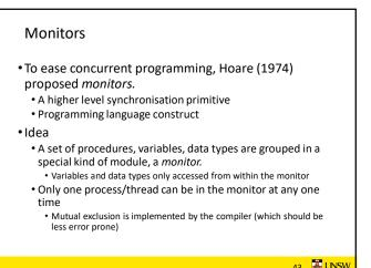
• When a thread calls a monitor procedure that has a thread already inside, it is queued and it sleeps until the current thread exits the monitor.
