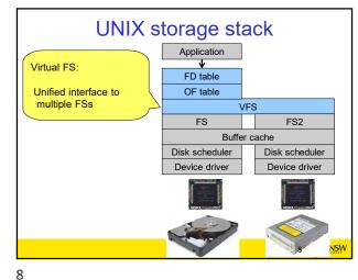
**UNIX storage stack** Application File desctriptor and Open file tables: FD table OF table Keep track of files VFS opened by user-level processes FS Buffer cache Matches syscall interface Disk scheduler to VFS Interface Device driver 9 🐺 UNSW
