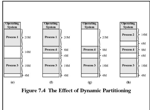
Figure 7.4 The Effect of Dynamic Partitioning
