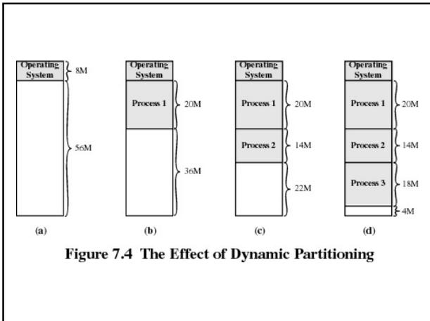
Figure 7.4 The Effect of Dynamic Partitioning
