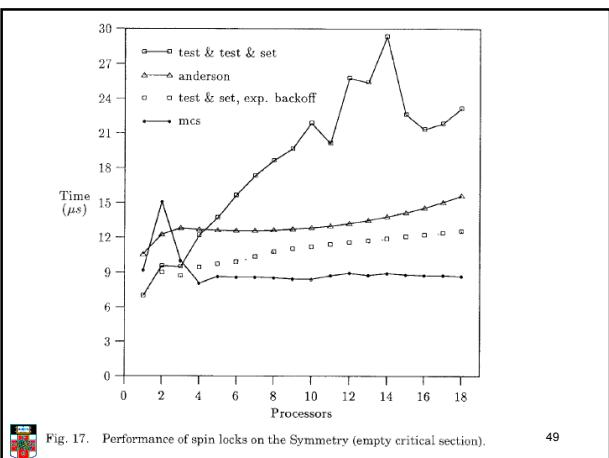
Fig. 17. Performance of spin locks on the Symmetry (empty critical section).
