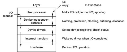
Layers of the I/O system and the main functions of each layer
