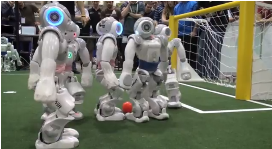
Fig. 33. rUNSWift vs. B-Human (3:4), RoboCup SPL 2012 Pool I. This photo illustrates the high incidence of robot's crowding the ball and tackling their own teammates during periods of wireless failure (rUNSWift in pink waist bands). In later games rUNSWift was able to mitigate this problem using the robot detection system.
