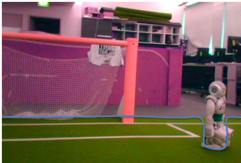
Fig. 28. Illustration of the concept of robot detection using field edge indents. No indent is shown around the goal post. Sourced from [21].
